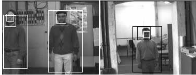
Figure 4. Example output frames from our system. The three bounding boxes are the object and head bounding boxes estimated by the motion-based tracker and the face detected in combination with the model-based face detector.
