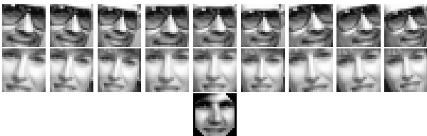
Figure 3. Examples of the face images used for training the neural network. The lower image shows the mask used.
