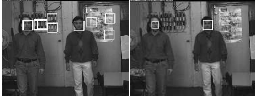
Figure 2. Left: Example output from a neural network based static face detector at a given scale. Erroneous detections occur due to “face-like” patterns. Right: Example output when the motion-based tracker and the model-based face detector are combined.
