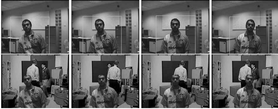
Fig. 5. Segmentation results. The top row outlines the tracked region for segmentation and the second row illustrates superimposition onto an alternative sequence.
