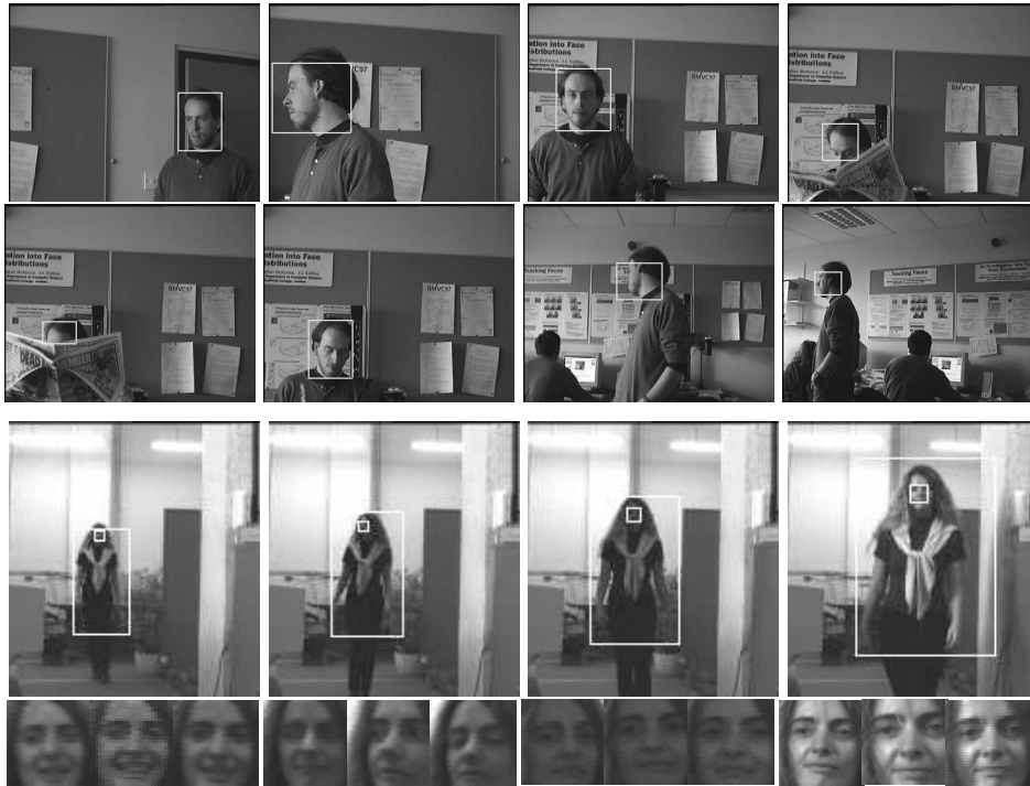
Figure 2: Real-time tracking and normalisation in dynamic scenes using colour, motion and neural nets based face appearance models. In the first sequence the system uses a colour model to cope with large pose variations and partial occlusion whilst the camera pans and zooms. In the second sequence, approximate body bounding boxes are also shown along with aligned and scale-normalised faces.
