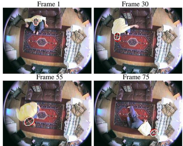
**Fig. 1.** Frames from a sequence in which the head is tracked using ILW. The person is tracked through a sudden fall. The white ellipse represents the most heavily weighted particle.
