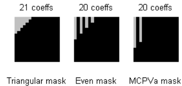
Fig. 5. Left to right; 21 coefficient ‘Tri’ mask, 20 coefficient ‘Even’ mask and 20 coefficient ‘MCPVa’ mask
